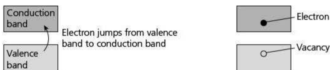
Figure 29.10 An electron jumps from the valence band to the conduction band, leaving a positive hole in the valence band
