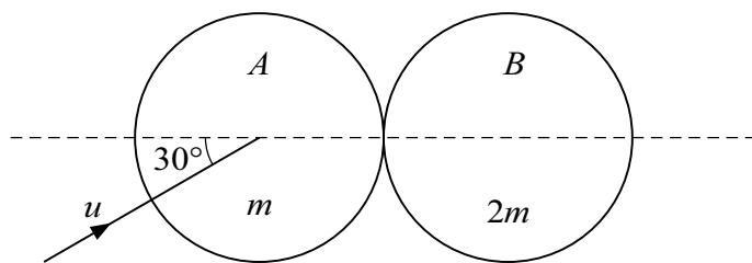
Two uniform smooth spheres  $A$  and  $B$  of equal radii have masses  $m$  and  $2m$  respectively. Sphere  $B$  is at rest on a smooth horizontal surface. Sphere  $A$  is moving on the surface with speed  $u$  at an angle of  $30^\circ$  to the line of centres of  $A$  and  $B$  when it collides with  $B$  (see diagram). The coefficient of restitution between the spheres is  $e$ .
