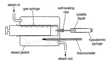
A known mass of volatile liquid is injected into the gas syringe using a hypodermic syringe. The injected volatile liquid vaporises and the volume of vapour is recorded.
