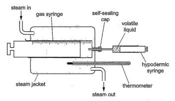
A known mass of volatile liquid is injected into the gas syringe using a hypodermic syringe. The injected volatile liquid vaporises and the volume of vapour is recorded.
