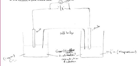
This diagram is incorrect. It should have shown a circuit with a voltmeter and without a cell. The metals should have been labelled and the concentrations of the solutions should have been stated as 1(.00) mol dm<sup>-3</sup>.
