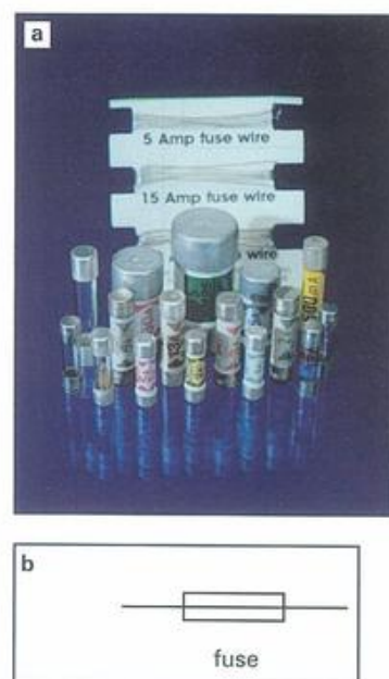
Figure 19.27 a Cartridge fuses and fuse wire. The thicker the wire, the higher the current that causes it to blow. b The circuit symbol for a fuse.
