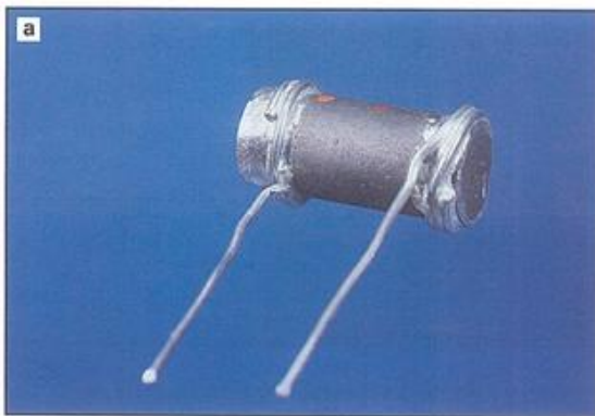
Figure 19.6 a A thermistor. b The resistance of a thermistor depends on the temperature. In this case, in the middle of the curve, its resistance drops a lot as the temperature increases by a small amount. c In the circuit symbol, the line through the resistor indicates that its resistance is not fixed but depends on an external factor (in this case, the temperature).
