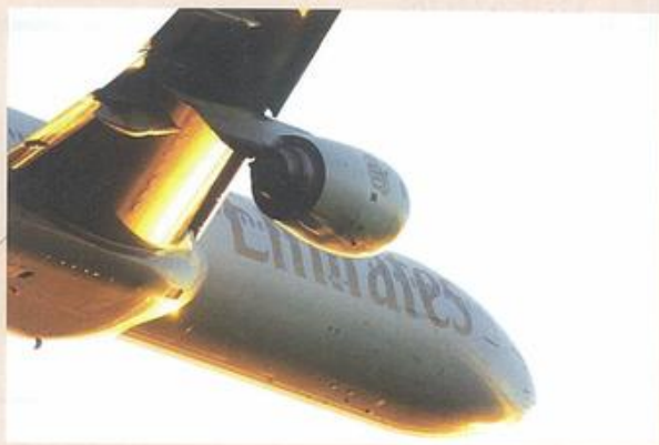
Figure 3.9 A jumbo jet has four engines, each capable of providing a quarter of a million newtons of thrust. When the aircraft lands, the engines are put into 'reverse thrust' mode, so that they provide a decelerating force to bring it to a halt.
