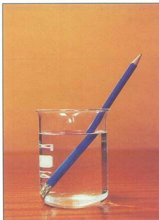
Figure 13.8 The pencil is partly immersed in water. Because of refraction of the light coming from the part of the pencil that is underwater, the pencil appears broken.
