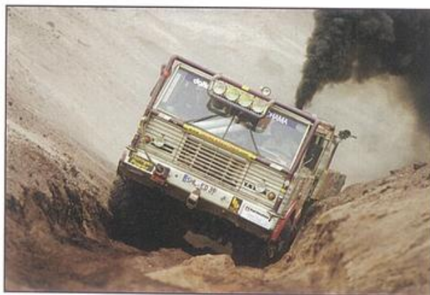
Figure 5.10 This truck has wide tyres to spread its weight as it travels over the sand dunes. Camels have big, flat feet for the same reason, to reduce the pressure on the sand so that they are less likely to sink in and become bogged down.
