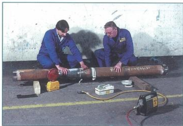
Figure 23.16 Checking for faults in a metal pipe. The engineers are checking that no radiation is escaping from the pipe. The gamma source is stored in the black box in the foreground, but can be pushed through the long tube along the pipe to reach the part to be checked.
