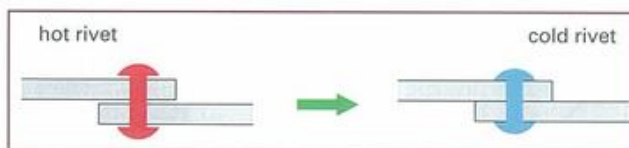
Figure 10.10 Joining two metal plates using a rivet.
