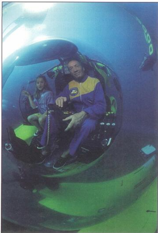
Figure 5.11 This underwater exploring vehicle is used to carry tourists to depths of 600 m, where the pressure is 60 times that at the surface. The design makes use of the fact that spherical and cylindrical surfaces stand up well to pressure. The viewing window is made of acrylic plastic and is 9.5 cm thick.
