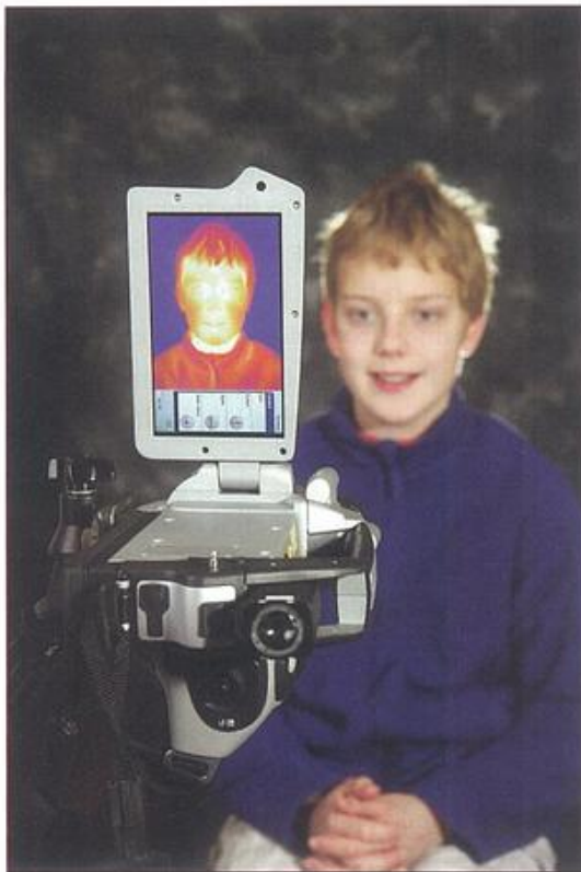
Figure 11.11 Using an infrared-sensitive camera. Slight variations in body temperature show up as different colours. Cameras like this are used in medicine to detect skin disorders and infections.
