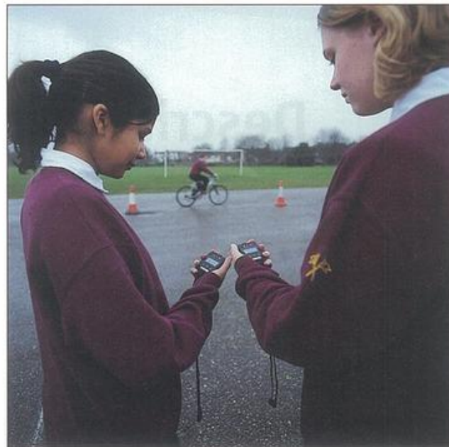
Figure 2.3 Timing a cyclist over a fixed distance. Using a stopwatch involves making judgements as to when the cyclist passes the starting and finishing lines. This can introduce an error into the measurements. An automatic timing system might be better.
