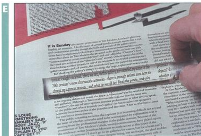
Figure 13.22 This long converging lens is designed to help people to read. It produces a magnified image of a line of print. The user simply slides it down the page.
