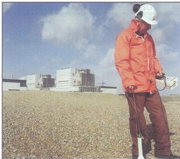
Figure 7.6 This nuclear power station generates electricity. Its fuel is uranium. As the fuel is used up, highly radioactive waste products are produced. These have to be dealt with very carefully to avoid harm to the surroundings. Here, checks are being carried out to ensure that the level of radioactive materials near the power station is safe.
