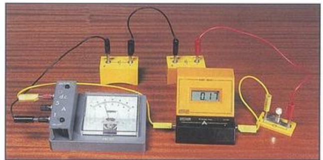
Figure 18.4 Ammeters measure electric current, in amps (A). There are two types: analogue (on the left) and digital (on the right).
