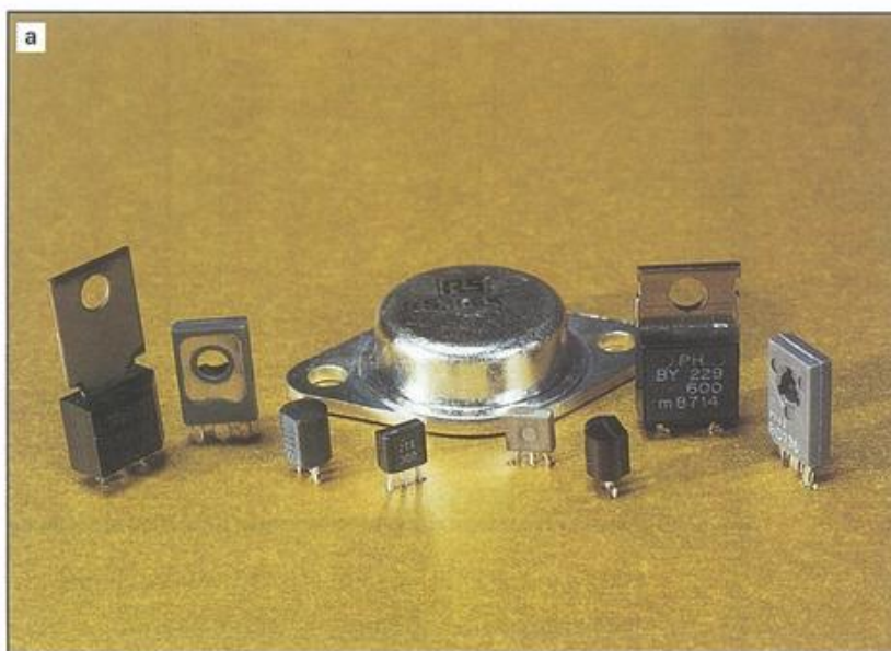
Figure 19.17 a Some transistors. b The circuit symbol for a transistor, along with the names of the three terminals. c With no current flowing into the base, no current can flow through the transistor. When a small current flows into the base, a large current flows into the collector, through the transistor and out through the emitter. (The arrows show the direction of current flow. The emitter emits electrons in the opposite direction to the flow of conventional current, and the collector collects them.)
