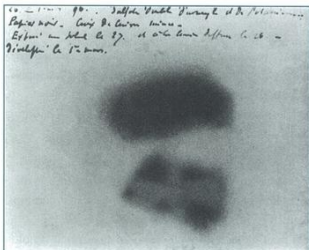
Figure 23.5 One of Henri Becquerel's first photographic records of the radiation produced by uranium. The two black blobs are the outlines of two crystals containing uranium. To show that the radiation would pass through metal, he placed a copper cross between one of the crystals and the photographic film. You can see the 'shadow' of the cross on the photograph. The writing is Becquerel's; the last line says 'développé le 1er mars' – developed on 1st March (1896).
