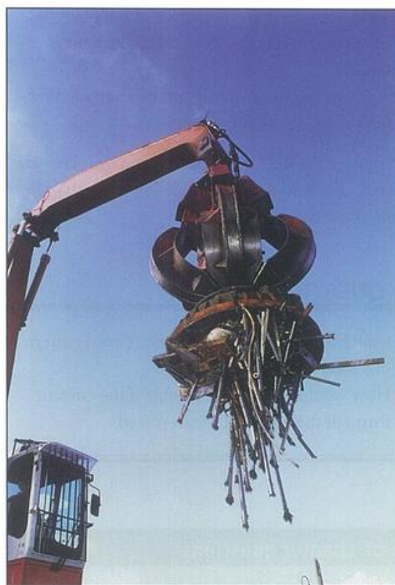
Figure 16.10 Using an electromagnet in a scrapyard. A steel object or pile of scrap can be lifted and moved. Then the current is switched off to release it.
