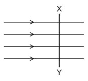
In which direction is the rod moved so that there is an induced current from Y to X?
