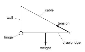
The weight of the drawbridge and the tension in the cable are represented by the labelled arrows in the diagram. There is a third force at the hinge, which is not shown. The drawbridge is in equilibrium.
