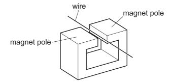
Which action does not induce an e.m.f. in the wire?
