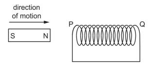
Magnetic poles are produced at the two ends of the coil as the magnet enters and as the magnet leaves the coil.
