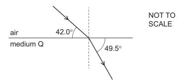
What is the critical angle for the boundary between medium Q and air?
