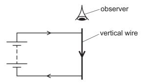
What is the pattern of the magnetic field around the wire seen by an observer viewing the wire from the position shown?
