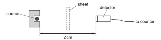
Counter readings are taken with and without sheets of different materials placed between the source and the detector.
