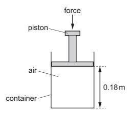
A force is applied to move the piston down into the container. The temperature of the air remains constant. The distance between the base of the container and the piston decreases from  $0.18\,\mathrm{m}$  to  $0.15\,\mathrm{m}$ .
