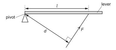
Length *d* is the perpendicular distance between the force and the pivot.
