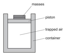
A mass of 1.0 kg is placed on the piston and the volume of the trapped air decreases from 100 cm<sup>3</sup> to 90 cm<sup>3</sup>.
