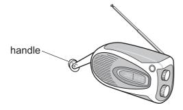
A person winds a spring in the radio using the handle. When the spring unwinds, it makes a small coil rotate in a magnetic field.
