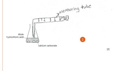
3 The 'measuring tube' has some syringe character in it (the plunger at the end), so benefit of the doubt is given for this part of the drawing, despite the incorrect label (candidates are not asked to label the apparatus). The second mark is not awarded because gas could escape from the flask: the system is not closed.
