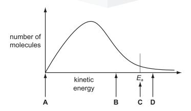
**32** The Boltzmann distribution below shows the distribution of molecular energies in a sample of a gas at a given temperature.
