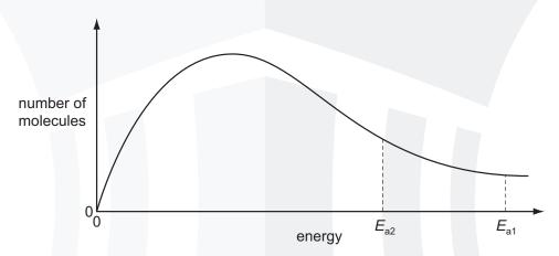
$E_a$  is the activation energy for the reaction between the gases. Of the two values shown, one is for a catalysed reaction, the other for an uncatalysed one.
