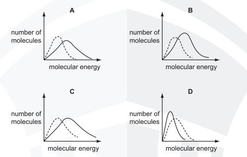
**31** The diagram below represents, for a given temperature, the Boltzmann distribution of the kinetic energy of the molecules in a mixture of two gases that react slowly together.
