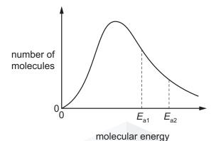
$E_{a}$  is used to represent the activation energy for the reaction between the gases. Of the two values shown, one is the activation energy for a catalysed reaction, the other for an uncatalysed reaction.
